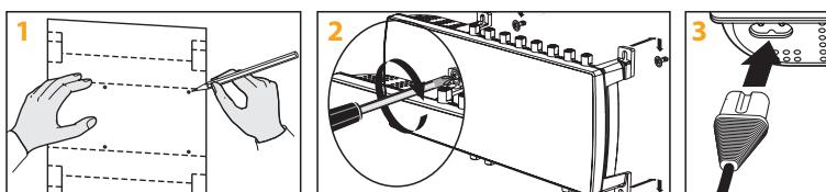
1 - Vertical installation (height ≤ 2 m) / Montaje vertical (altura ≤ 2 m)
